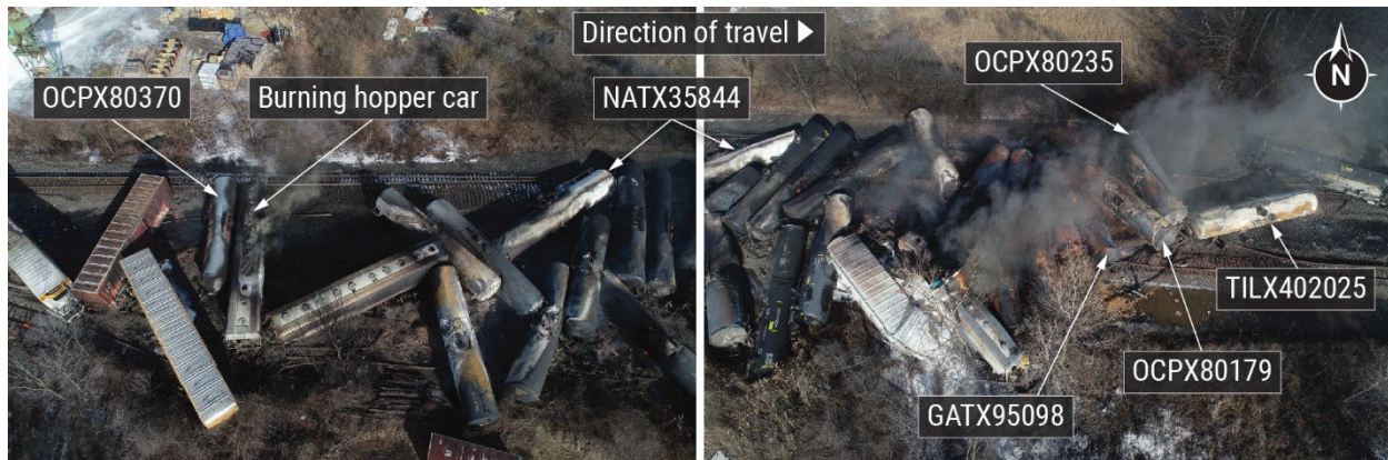
Figure 7. Derailment pileup and VCM tank cars.
