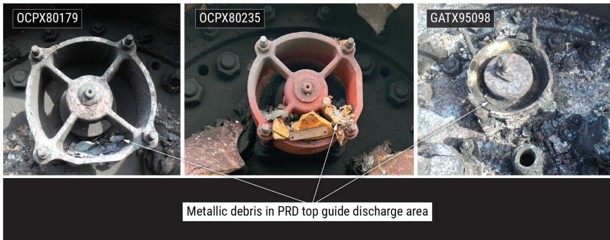
Figure 22. Metallic debris in the PRDs of tank cars equipped with aluminum protective housing covers.
