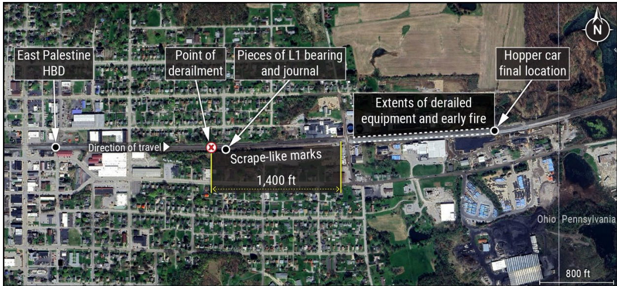
Figure 28. Locations of derailment evidence.
