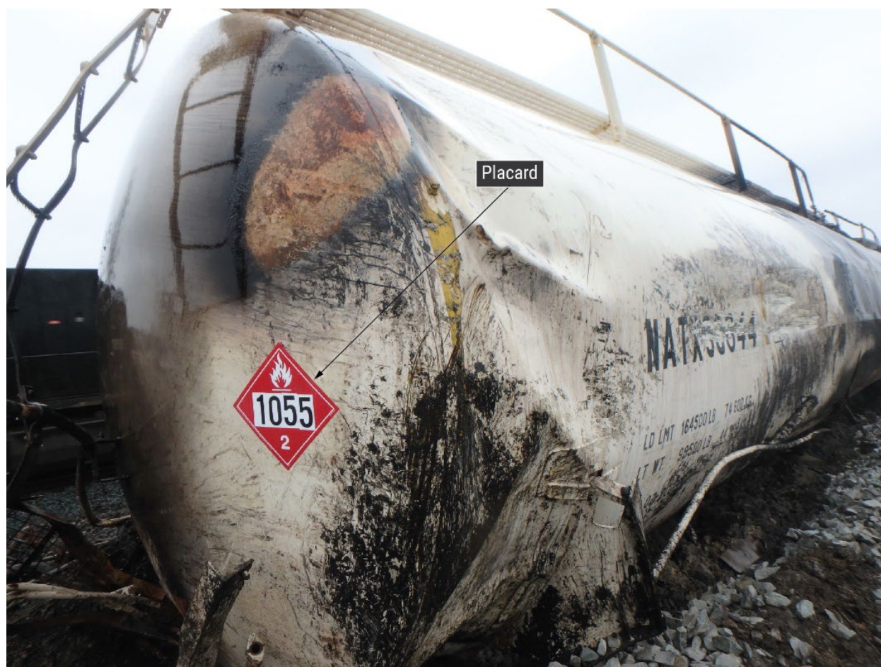
Figure 25. Replacement placard on a derailed DOT-105 tank car containing isobutylene.
